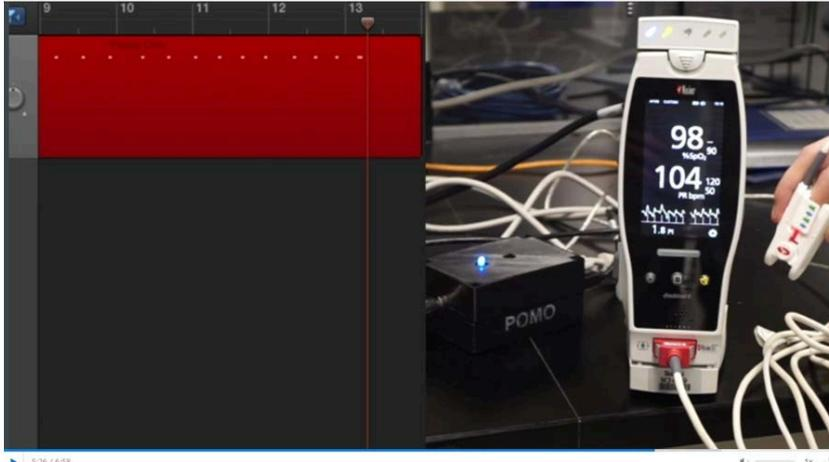
*Figure 1: POMO Device outputting in real-time from pulse-oximeter to GarageBand*
